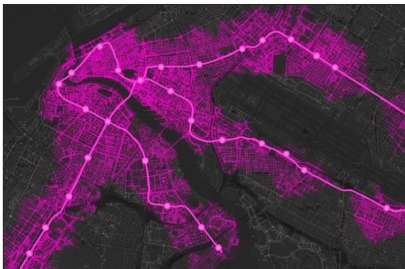
Accessibility of Dubai's metro stations (20-minute-walking and 8-minute-cycling radius), source: Own figure, OSM data
